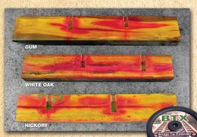
The penetration of borates into the wood is indicated by the red coloring of added curcumin.
